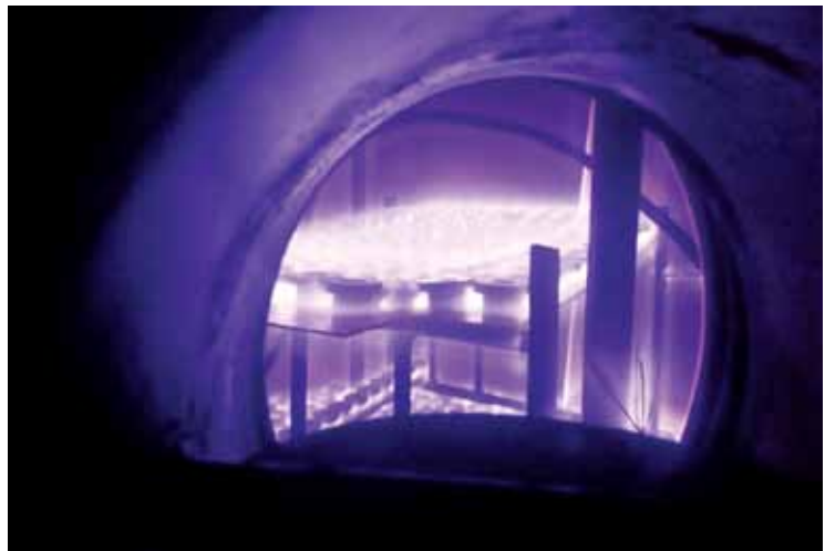
Environmental Friendly Technology-Improvement in wear resistance by Plasma Nitriding
